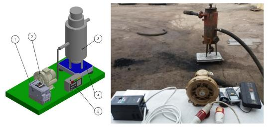
Fig. 1. **Experimental plant:** 1 – frequency converter Hitachi-3G3JX-A4075-EF; 2 – blower Goorui GHBH-0D5-34-1R2; 3 – downdraft gasifier; 4 – weight scales; 5 – weight scales indicator
